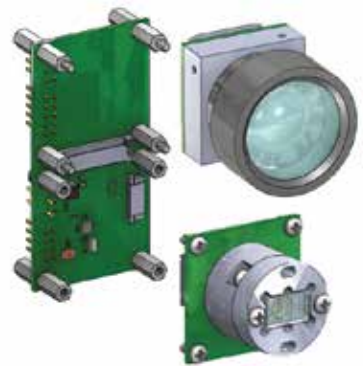
The laser (emitter), lens (receiver) and carrier board can be integrated as modular entities with LeddarVu.
